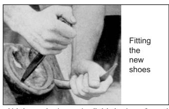
which the new shoe is to rest is called the bearing surface, and if this is not quiet leveled, then the horn will be seared by the hot shoe more at one point than another. Here again the necessary adjustments can now be made with the rasp.
