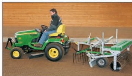
Platz-Max Auto SF – a very good and manoeuvrable team for levelling, but also multifunctional use for mowing, sweeping, transporting etc. A hydraulic track-clearer is attached to the towing vehicle.
