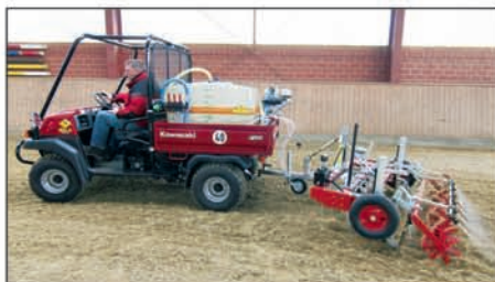
Platz-Max Roll – with optional "Rain-Module": flexible system for any towing vehicles with a little loading space for the water tank. Special appliances allow diverse other vehicles also carrying a tank, too.
