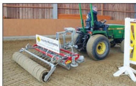
Platz-Max FFW – with swivelling mechanism and special heavy roller to loose, mix up, level and harden the surface again, especially used to maintain the variety of different jumping-grounds
