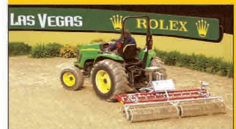
Platz-Max NL-GW Plus – with swivelling mechanism, on duty during the World Cup Finals Las Vegas 2009 with lattice roller divided in two parts.
