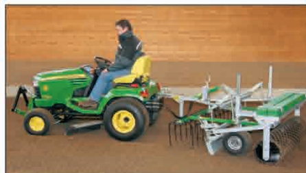
Platz-Max Auto SF – a very good and manoeuvrable team for levelling, but also multifunctional use for mowing, sweeping, transporting etc. A hydraulic track-cleaver is attached to the towing vehicle.
