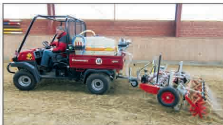
Platz-Max Roll – with optional "Rain-Module": flexible system for any towing vehicles with a little loading space for the water tank. Special appliances allow diverse other vehicles also carrying a tank, too.
