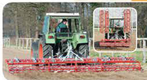
"Platz-Max Turf" – especially developed for the use on large race courses, where a quick smoothing between several horse-racings is required. Folding by hydraulic.
