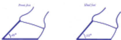
Side view of the foot axis The foot axis and the angle of the wall at the heels should correspond and be between 45 & 50 degrees.
