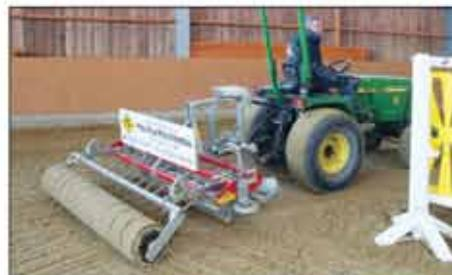
Platz-Max FFW – with swivelling mechanism and special heavy roller to loose, mix up, level and harden the surface again, especially used to maintain the variety of different jumping-grounds
