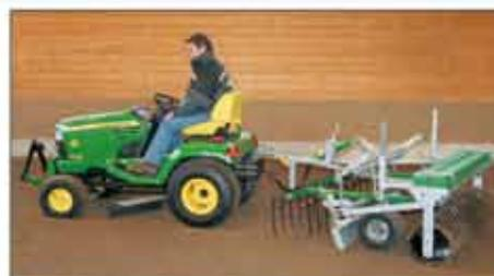
Platz-Max Auto SF – a very good and manoeuvrable team for levelling, but also multifunctional use for mowing, sweeping, transporting etc. A hydraulic track-cleaver is attached to the towing vehicle.
