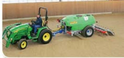
**The Platz-Max Giga** – for fast levelling and watering large and little riding areas. Very manoeuvrable by special connection to the tractor. 2 hydraulic levelling units, 4 rows of water sprayers to switch on/off separately (up to 180 l/min.), 3 sizes of water tanks and lot of extras.
