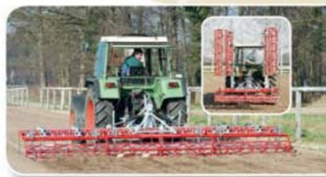
**The Platz-Max Turf** – especially developed for the use on large race courses, where a quick smoothing between several horse-racings is required. Folding by hydraulic.
