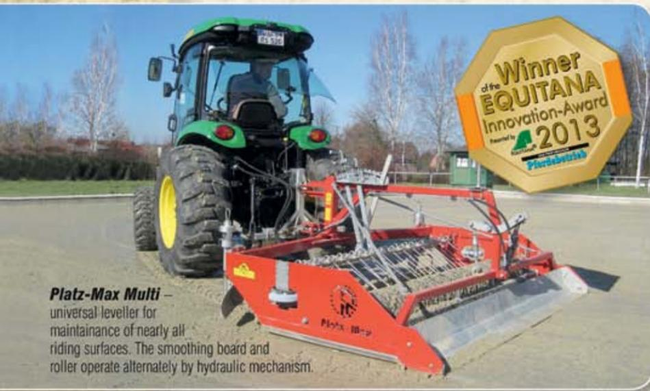
**Platz-Max Multi** – universal leveller for maintenance of nearly all riding surfaces. The smoothing board and roller operate alternately by hydraulic mechanism.
